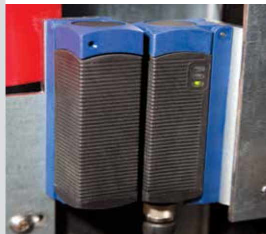
Class 4 safety switches verify closure
