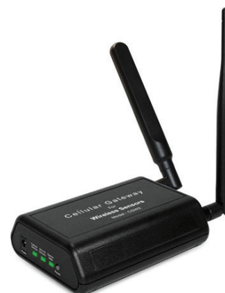
Wireless cellular Gateway receives signal that door was hit
